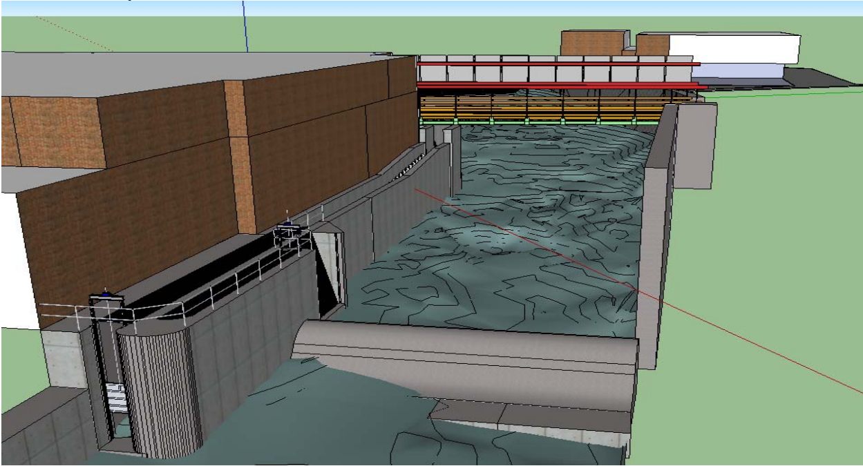
Slide -13 Phase 2 Freshet Channel Depicted View Looking Upstream in the Freshet Channel (Denil Fishway Entrance, Attraction Flow Intake and Barrier Dam)
